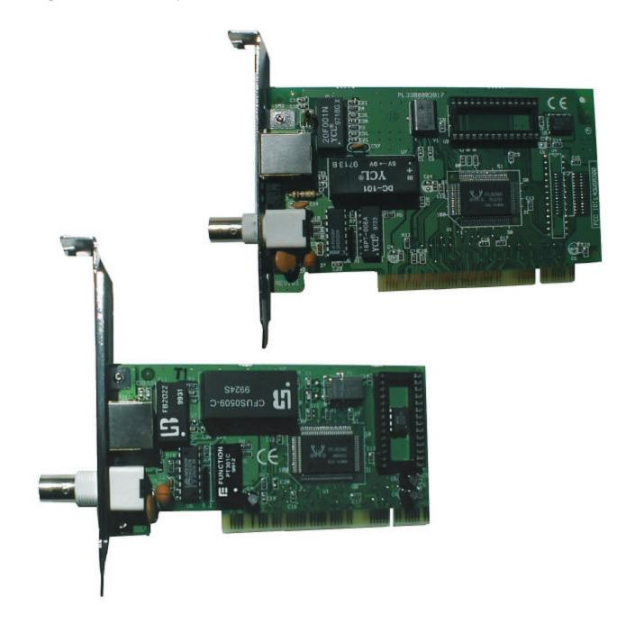
Adapter Name: Noderunner Pro Drivers DOS: NPRO.EXE NPRO.EXE Win 3.x: Win 95: Intel EtherExpress Pro/10 Win 98: Intel 82595-based Ethernet Intel EtherExpress Pro Ethernet Adapter Win NT: Setup utility: NPROSET.EXE NPROSET.EXE Diagnostic: How to Identify We sell a Combo version (with BNC and RJ-45 jacks) and a UTP version (with only the RJ-45 jack).
