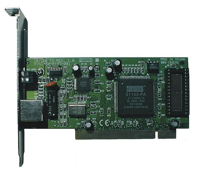
Adapter Name: i.Share Ethernet Starter Kit Adapter (aka PCI 10Mbps Combo Adapter) Manufacturer: NDC Model Number: ND4300 Drivers DOS: ND4300.EXE Win 3.x: ND4300.EXE Win 95: Artisoft ND4300 Ethernet Adapter Win 98: Artisoft ND4300 Ethernet Adapter Win NT: Artisoft ND4300 Ethernet Adapter Setup utility: NDCDIAG.EXE Diagnostic: NDCDIAG.EXE How to Identify There are two revisions of this adapter, and they are very different in appearance.
