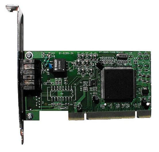
Adapter Name: Fast Ethernet Starter Kit adapter Manufacturer: KTI KF-230TX/2 Model Number: Drivers DOS: RTSLAN5.EXE Win 3.x: RTSLAN5.EXE Win 95: KF-230TX Fast Ethernet PCI Adapter Win 98: KF-230TX Fast Ethernet PCI Adapter KF-230TX Fast Ethernet PCI Adapter Win NT: Setup utility: SETUP.EXE Diagnostic: SETUP.EXE How to Identify This is a PCI adapter. In the upper left corner (near the silver edge bracket) it indicates 10/100TX
